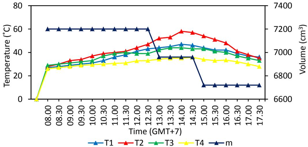
Figure 7. Relationship of temperature and water evaporation rate of type-II solar distillation
