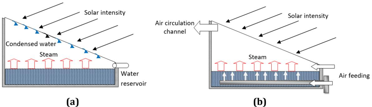
Figure 3. Schematic of the work process of testing (a) type-I and (b) type-2 solar distillation
