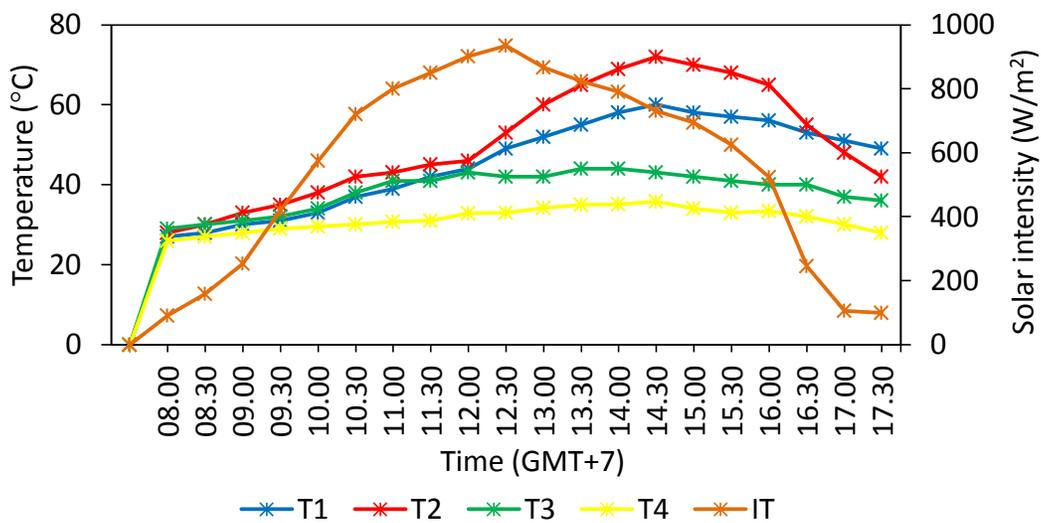
Figure 4. Relationship between temperature and solar intensity type-I solar distillation
