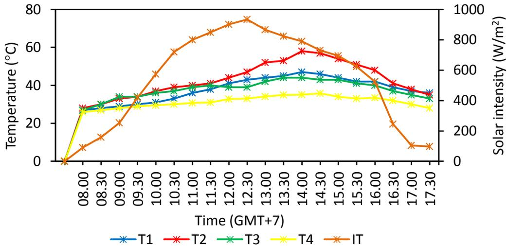
Figure 5. Relationship between temperature and solar intensity type-II solar distillation
