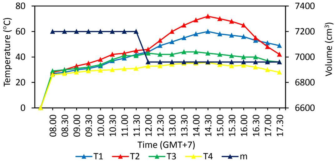
Figure 6. Relationship of temperature and evaporation rate of type-I solar distillation
