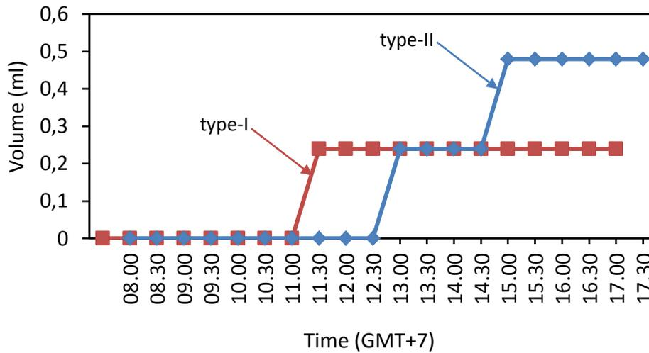
Figure 8. Comparison of vapor volume production in type-I and type-II solar distillation
