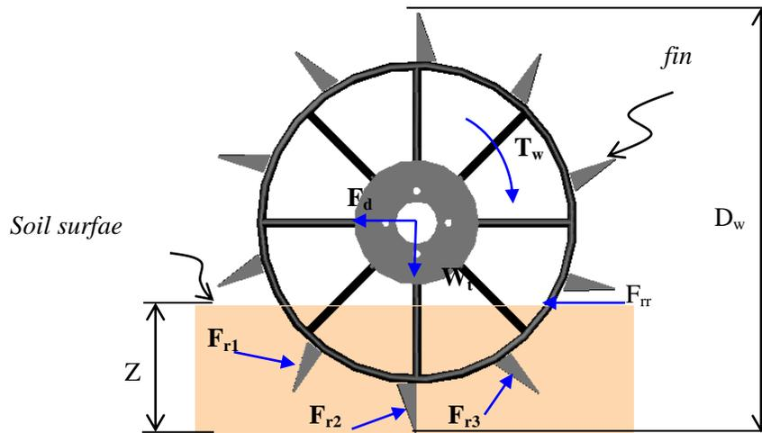
Figure 2 A force scheme that acts on the cage wheel for wheel design parameters
