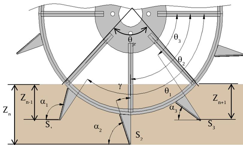
Figure 4 Position scheme and lugs angle of of tractor wheels
