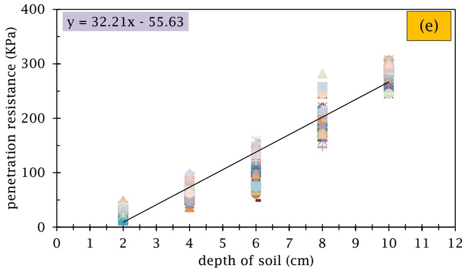
Figure 5 Graph of soil depth vs pressure resistance (a) pressure angle 30° (b) pressure angle 45° (c) pressure angle 60° (d) pressure angle 75° (e) pressure angle 90°
