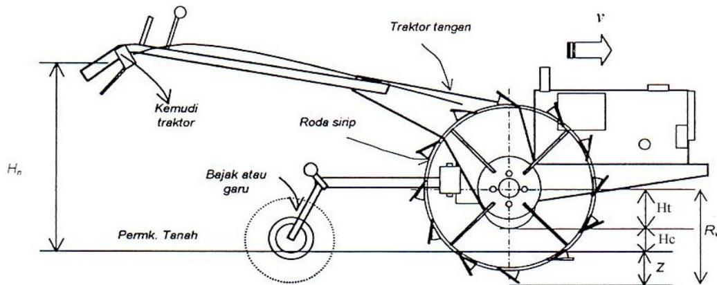
Figure 3 The basic formation of hand tractors in Indonesia
