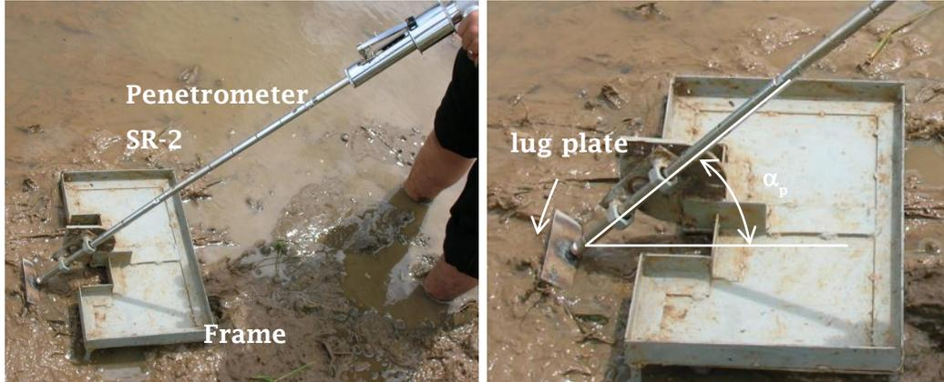
Figure 1 Penetrometer and penetrometer frame, penetration resistance measurement method
