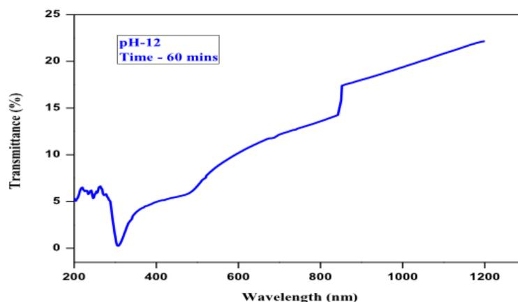
Figure 2. Transmittance Spectrum of CdS thin films prepared at pH 12 (60 minutes)
