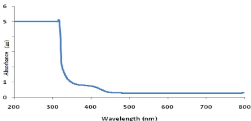
Figure 3. UV Visible absorbance Spectra of Zinc doped CdS thin films prepared at pH 12 (60 minutes)
