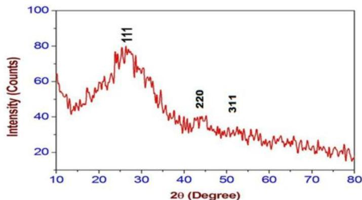
Figure 1. X-ray Diffraction spectra of Zinc doped CdS thin films prepared at pH 12 (60 minutes)
