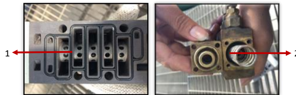
1. Solenoid directional valve; 2. Directional limit switch
